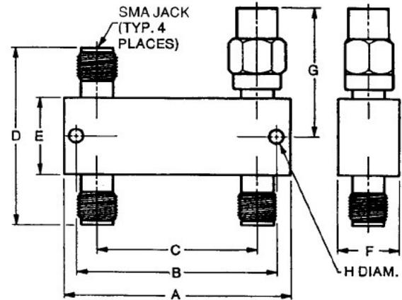
NOTE: All dimensions are  $\pm .020$ , except mounting hole diameters ( $\pm .005$ ) and mounting hole location ( $\pm .010$ ).
